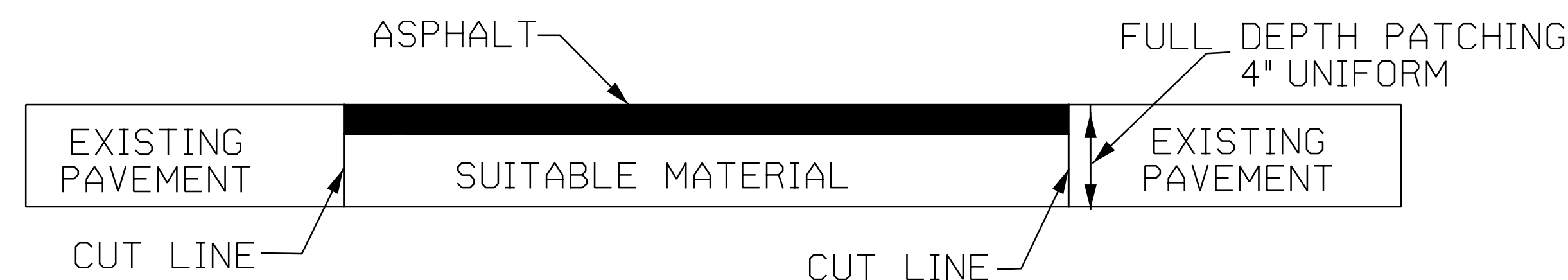
DETAIL OF FULL DEPTH PATCHING
